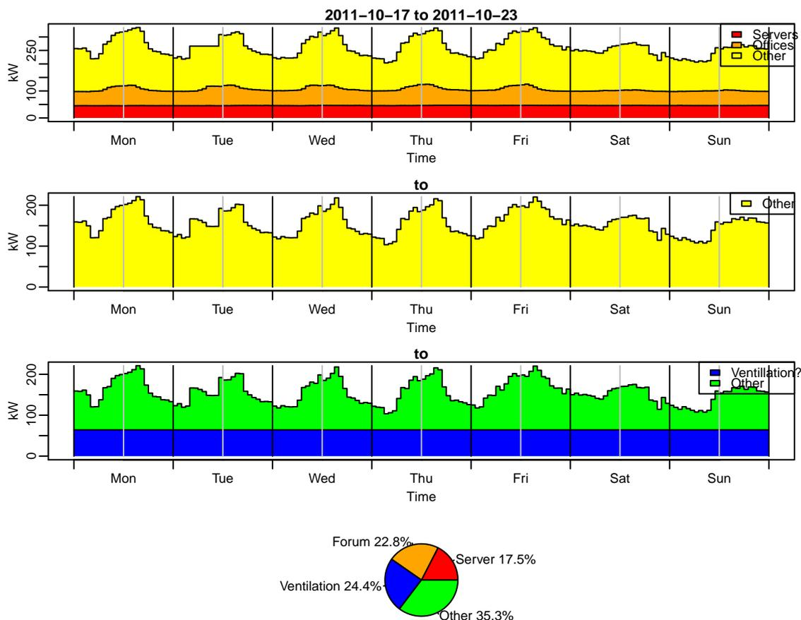
Figure 1: Hourly energy use in a term-time week in the Informatics Forum. **Top:** Total energy use, separated into components for servers, Forum offices and “other” use. **2nd graph:** Expanded view of the “other” energy use. **3rd graph:** “Other” decomposed into an inferred component for ventilation, and a remaining “other”. **Pie chart:** Share of energy use of the four components: “Forum” means “Offices” in this chart.
