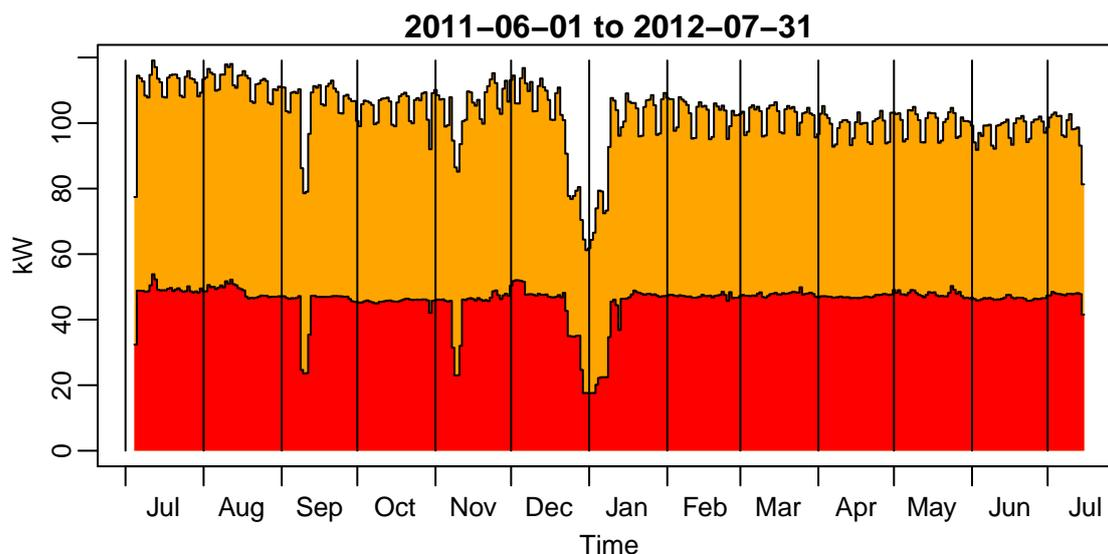
Figure 3: Energy use by servers (red) and computers and other appliances in offices (orange). Note that some of the dips in the server date (particularly in the Christmas vacation) are due to loss of data from the UPS rather than machines being turned off, though some servers were turned off in the vacation.
